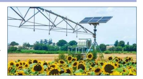
Solar energy is converted into electricity via photovoltaic panels installed on the central unit. The orientation and the tilt of the panels are adjustable to optimize energy production. The energy produced is stored on batteries which supply the electricity to power the pivot.
