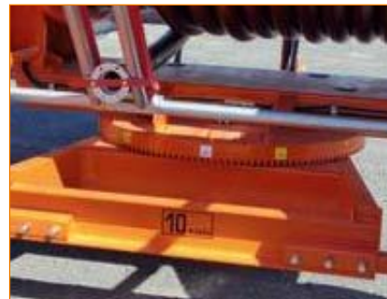
Hydraulic rotation of the turntable
