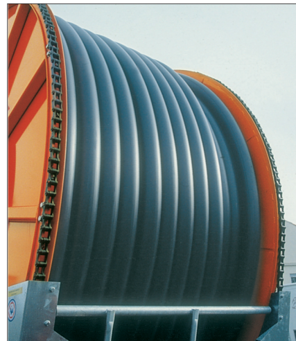
Twin drum drive chains
