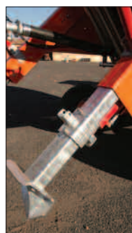
Hydraulic stabilisers and rotation of the turntable
