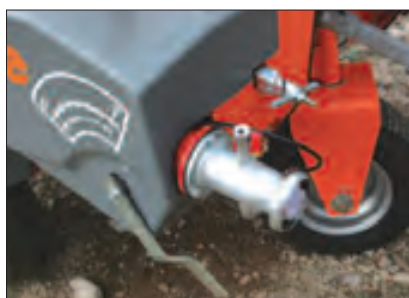
Speed regulation through by-pass
