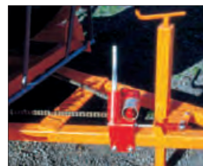
Mechanical jack and rotation of the turntable
