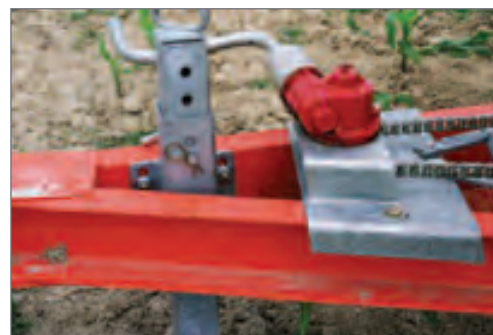
Automatic trolley lifting preventing crop-washing damages
