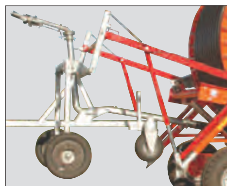
Lifting of the trolley connected to the hydraulic lifting of the stabilizers (Premium type)
