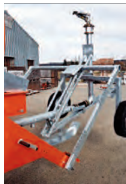
Automatic trolley lifting preventing crop-washing damages
