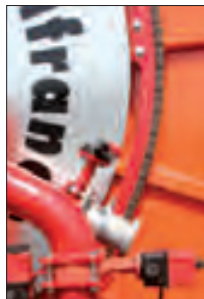
Rack and chain drive reel
