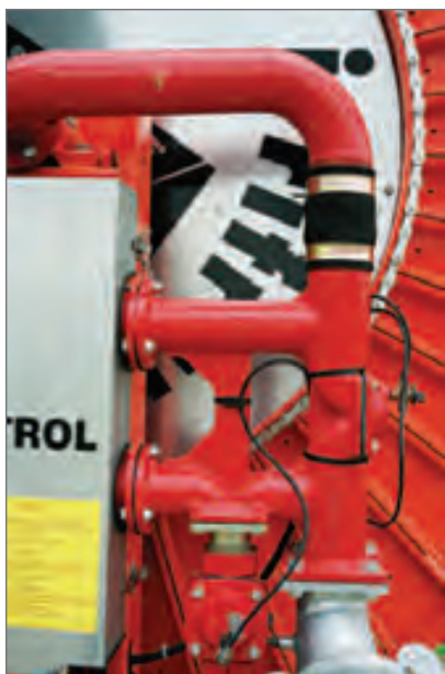
Supply tubing with integrated valve
