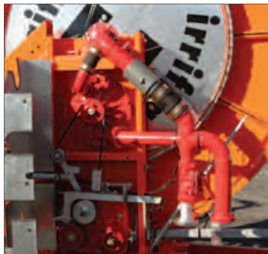
Automatic shut-off valve or discharge valve
