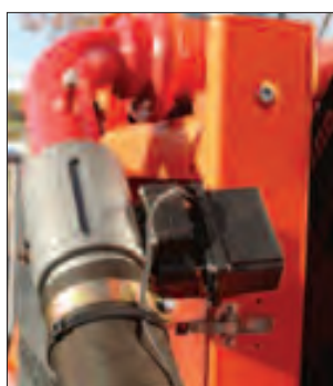
Butterfly valve controlled by electric motor
