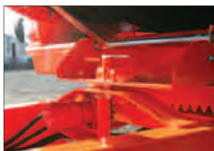
Hydraulic rotation of the turntable
