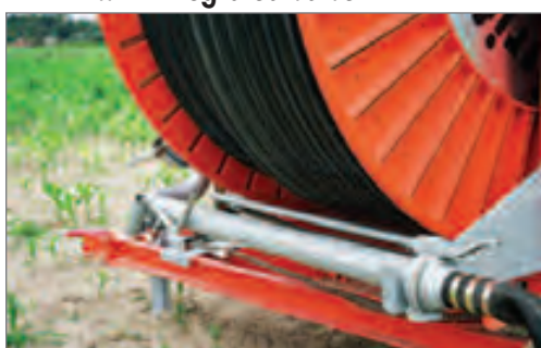
Supply tubing with integrated valve
