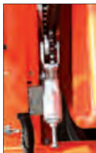
Rack and chain drive reel
