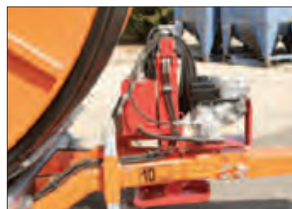
Rack and chain drive reel
