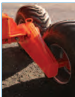
Articulated tandem axle (adjustable track)
