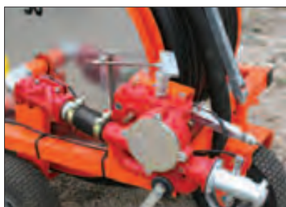
Low-pressure turbine drive
