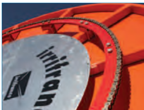
Chain and pinion drive
