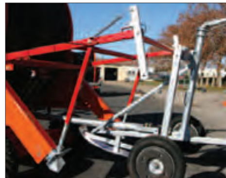
Hydraulic lifting connected to the lifting of the stabilizers (Premium type)
